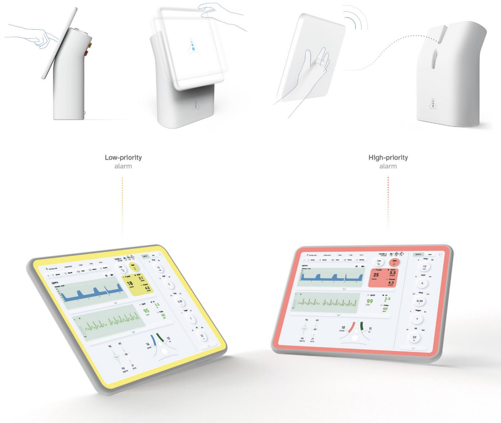
Figure 4. Reclinable and removable tablet to facilitate the reading and adjustment of ventilation parameters (top) and digital interface of the new ventilator, which communicates detected issues to the user through visual and auditory feedback (bottom).
